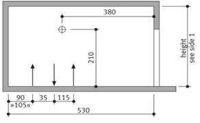
Units are dowelled to the floor. Drilling depth: approx. 15 cm. Floor and walls are to be made of concrete (quality minimum C20/25)!
