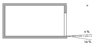
The illustrated maximum approach angles must not be exceeded. Incorrect approach angles will cause serious maneouvring & positioning problems on the parking system for which the local agency of SWISS-PARK accepts no responsibility.
